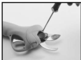
1. Disassemble the screws with a screwdriver and open the lid.
