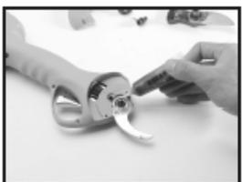
6. When replacing the blades, lubricating oil needs to be added between the blades
