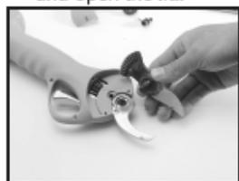
4. Disassemble the pin and remove the moving blade
